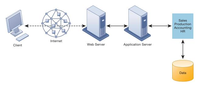
In a multitiered client/server network, client requests for service are handled by different levels of servers.
