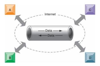
This VPN is a private network of computers linked using a secure tunnel connection over the Internet. It protects data transmitted over the public Internet by encoding the data and wrapping them within the Internet protocol. By adding a wrapper around a network message to hide its content, organizations can create a private connection that travels through the public Internet.
