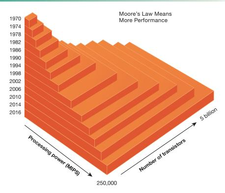
Packing more than 5 billion transistors into a tiny microprocessor has exponentially increased processing power. Processing power has increased to more than 250,000 MIPS (about 2.6 billion instructions per second).
