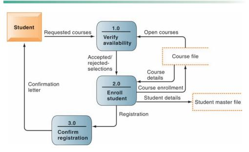
The system has three processes: Verify availability (1.0), Enroll student (2.0), and Confirm registration (3.0). The name and content of each of the data flows appear adjacent to each arrow. There is one external entity in this system: the student. There are two data stores: the student master file and the course file.
