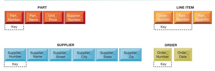
After normalization, the original relation ORDER has been broken down into four smaller relations. The relation ORDER is left with only two attributes, and the relation LINE\_ITEM has a combined, or concatenated, key consisting of Order\_Number and Part\_Number.
