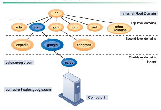
Domain Name System is a hierarchical system with a root domain, top-level domains, second-level domains, and host computers at the third level.
