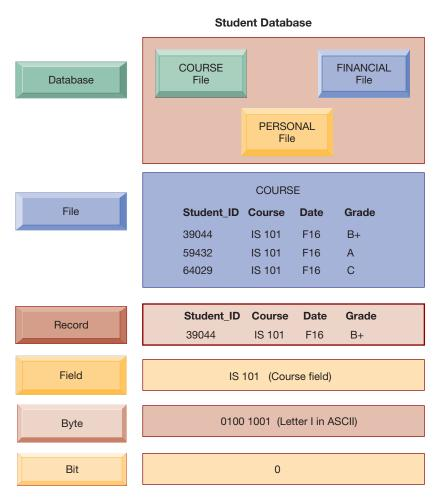
A computer system organizes data in a hierarchy that starts with the bit, which represents either a 0 or a 1. Bits can be grouped to form a byte to represent one character, number, or symbol. Bytes can be grouped to form a field, and related fields can be grouped to form a record. Related records can be collected to form a file, and related files can be organized into a database.
