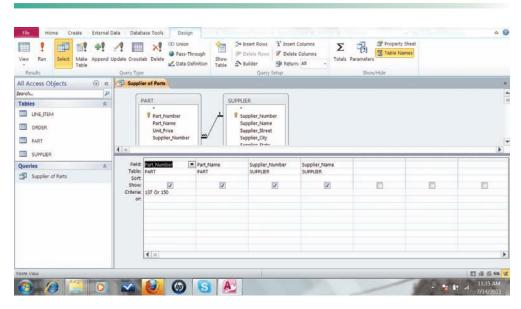
Illustrated here is how the query in Figure 6.7 would be constructed using Microsoft Access query-building tools. It shows the tables, fields, and selection criteria used for the query.
