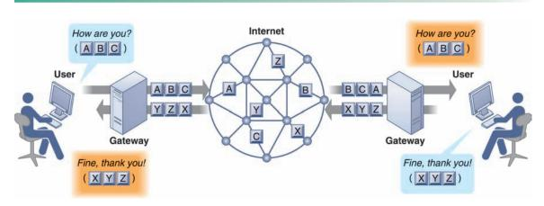
A VoIP phone call digitizes and breaks up a voice message into data packets that may travel along different routes before being reassembled at the final destination. A processor nearest the call's destination, called a gateway, arranges the packets in the proper order and directs them to the telephone number of the receiver or the IP address of the receiving computer.
