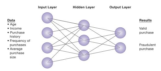
A neural network uses rules it "learns" from patterns in data to construct a hidden layer of logic. The hidden layer then processes inputs, classifying them based on the experience of the model. In this example, the neural network has been trained to distinguish between valid and fraudulent credit card purchases.
