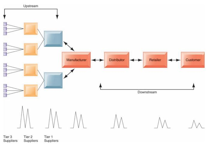
Inaccurate information can cause minor fluctuations in demand for a product to be amplified as one moves further back in the supply chain. Minor fluctuations in retail sales for a product can create excess inventory for distributors, manufacturers, and suppliers.
