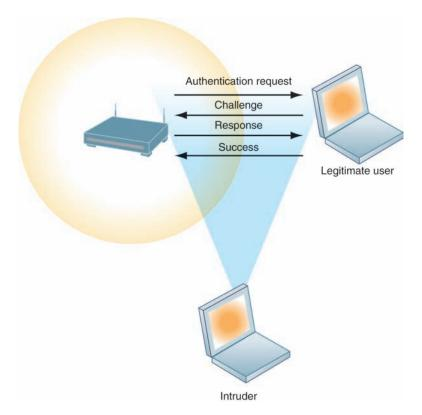
Many Wi-Fi networks can be penetrated easily by intruders using sniffer programs to obtain an address to access the resources of a network without authorization.
