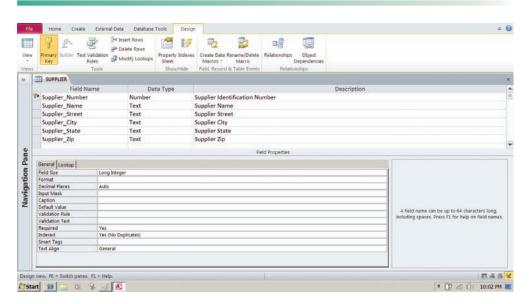
Microsoft Access has a rudimentary data dictionary capability that displays information about the size, format, and other characteristics of each field in a database. Displayed here is the information maintained in the SUPPLIER table. The small key icon to the left of Supplier\_Number indicates that it is a key field.
