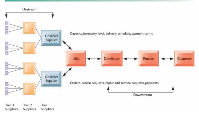
This figure illustrates the major entities in Nike's supply chain and the flow of information upstream and downstream to coordinate the activities involved in buying, making, and moving a product. Shown here is a simplified supply chain, with the upstream portion focusing only on the suppliers for sneakers and sneaker soles.
