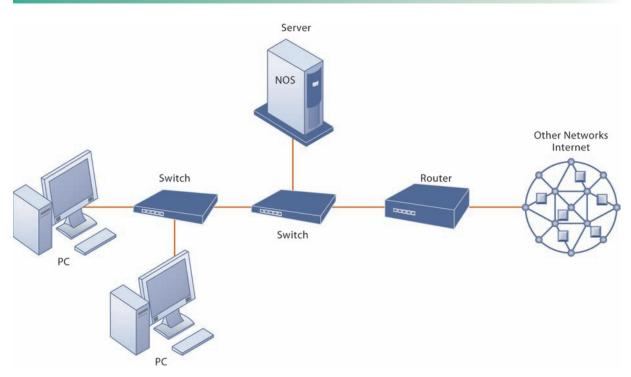
FIGURE 7.1 COMPONENTS OF A SIMPLE COMPUTER NETWORK
