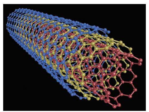
Nanotubes are tiny tubes about 10,000 times thinner than a human hair. They consist of rolled-up sheets of carbon hexagons and have potential use as minuscule wires or in ultrasmall electronic devices and are very powerful conductors of electrical
