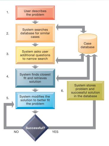
Case-based reasoning represents knowledge as a database of past cases and their solutions. The system uses a six-step process to generate solutions to new problems encountered by the user.
