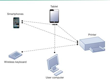
Bluetooth enables a variety of devices, including cell phones, smartphones, wireless keyboards and mice, PCs, and printers, to interact wirelessly with each other within a small, 30-foot (10-meter) area. In addition to the links shown, Bluetooth can be used to network similar devices to send data from one PC to another, for example.
