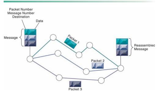
Data are grouped into small packets, which are transmitted independently over various communica-
