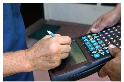
Using a handheld computer called a Delivery Information Acquisition Device (DIAD), UPS drivers automatically capture customers' signatures along with pickup, delivery, and time card information. UPS information systems use these data to track packages while they are being transported.
