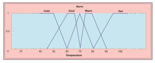
The membership functions for the input called temperature are in the logic of the thermostat to control the room temperature. Membership functions help translate linguistic expressions such as warm into numbers that the computer can manipulate.
