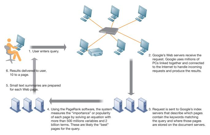
The Google search engine is continuously crawling the web, indexing the content of each page, calculating its popularity, and storing the pages so that it can respond quickly to user requests to see a page. The entire process takes about half a second.
