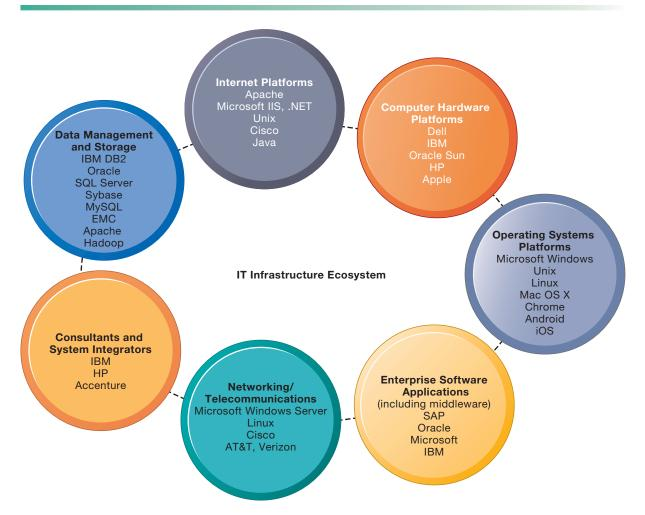
There are seven major components that must be coordinated to provide the firm with a coherent IT infrastructure. Listed here are major technologies and suppliers for each component.
