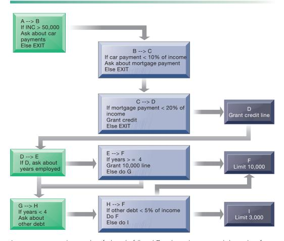
An expert system contains a number of rules to be followed. The rules are interconnected, the number of outcomes is known in advance and is limited, there are multiple paths to the same outcome, and the system can consider multiple rules at a single time. The rules illustrated are for simple credit-granting expert systems.
