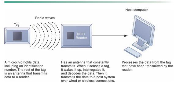
RFID uses low-powered radio transmitters to read data stored in a tag at distances ranging from 1 inch to 100 feet. The reader captures the data from the tag and sends them over a network to a host computer for processing. those data with other applications. Major enterprise software vendors now offer RFID-ready versions of their supply chain management applications.
