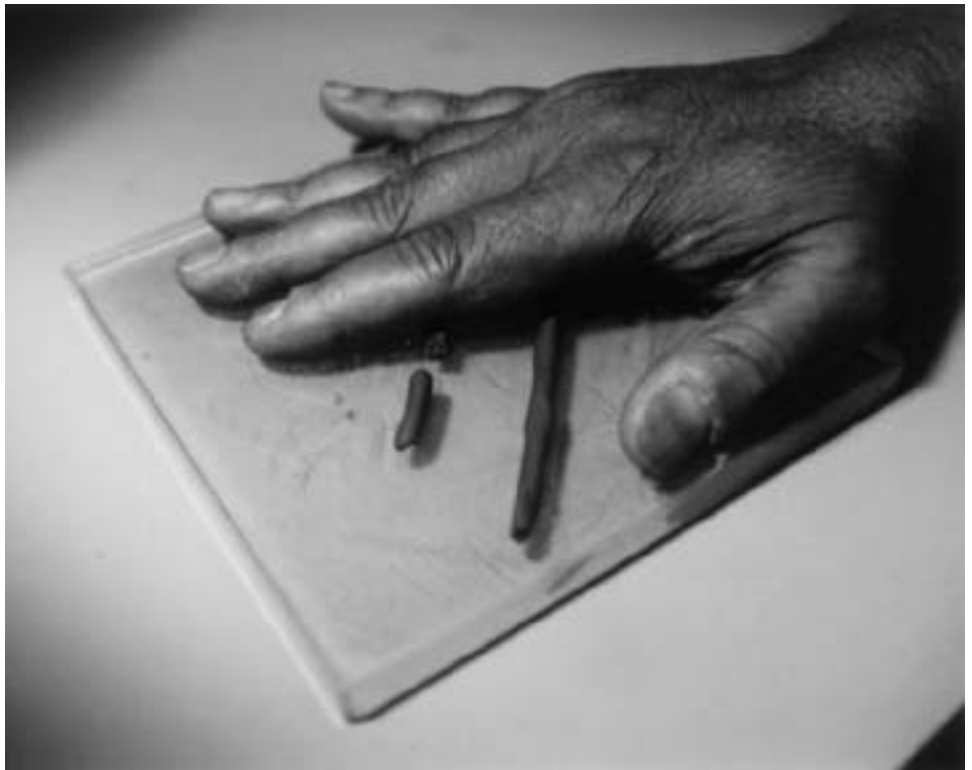
Figure 3.12 Plastic limit test (Courtesy of Braja Das)
