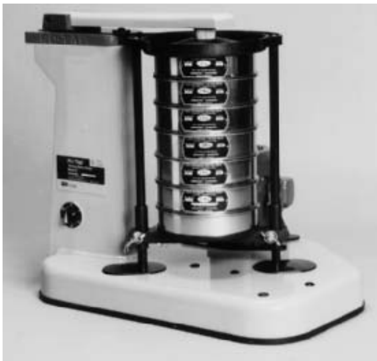
Figure 2.10 A set of sieves for a test in the laboratory (Courtesy of Braja Das)
