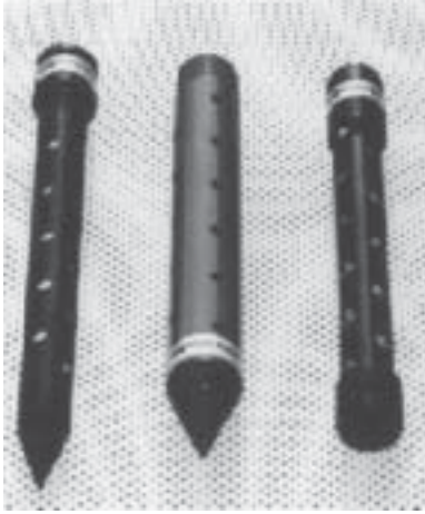
Figure 10.9 Components of a Casagrande-type piezometer (Courtesy of N. Sivakugan, James Cook University, Australia)
