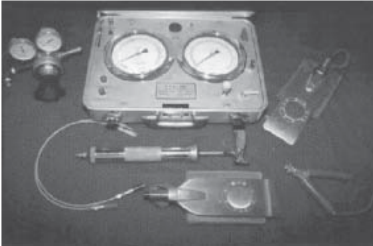
Figure 10.23 Assembly of equipment for dilatometer test (Courtesy of N. Sivakugan, James Cook University, Australia)
