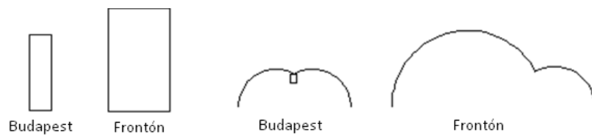
Figure 29: Size comparison in plan between the Frontón and Budapest shells and Directrix comparison between the same both structures.
