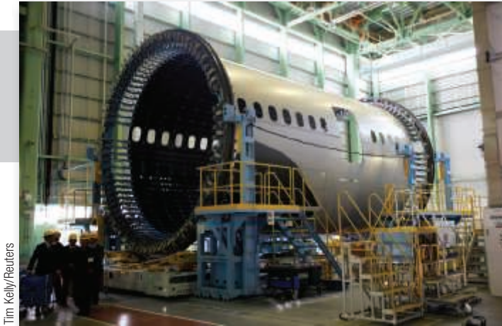
State-of-the-art composite sections of the 787 are built around the world and shipped to Boeing for final assembly.
